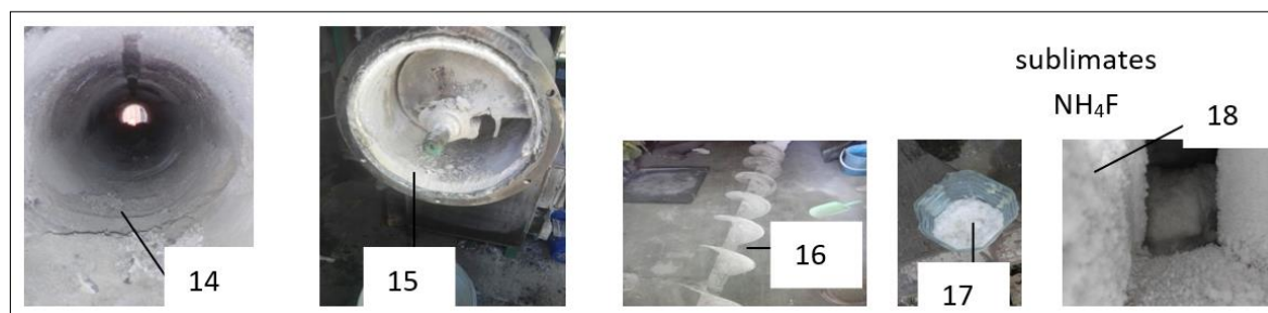
Fig 2: After testing: 14-garnissage; 15-charge and sublimes from the side of the bunker; 16-screw; 17-sublimes from the condenser; 18 - sublimes in an empty bunker for charge
